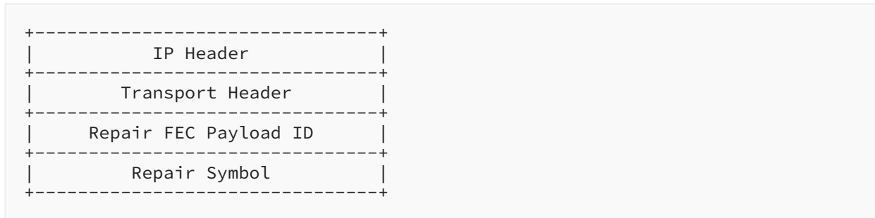
Figure 7: Structure of an FEC Repair Packet with the Repair FEC Payload ID
